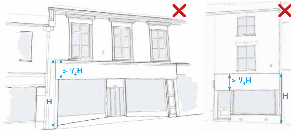
Loss of original features with the addition of a large sign. Oversailing the fascia, pilasters, and window heads.
