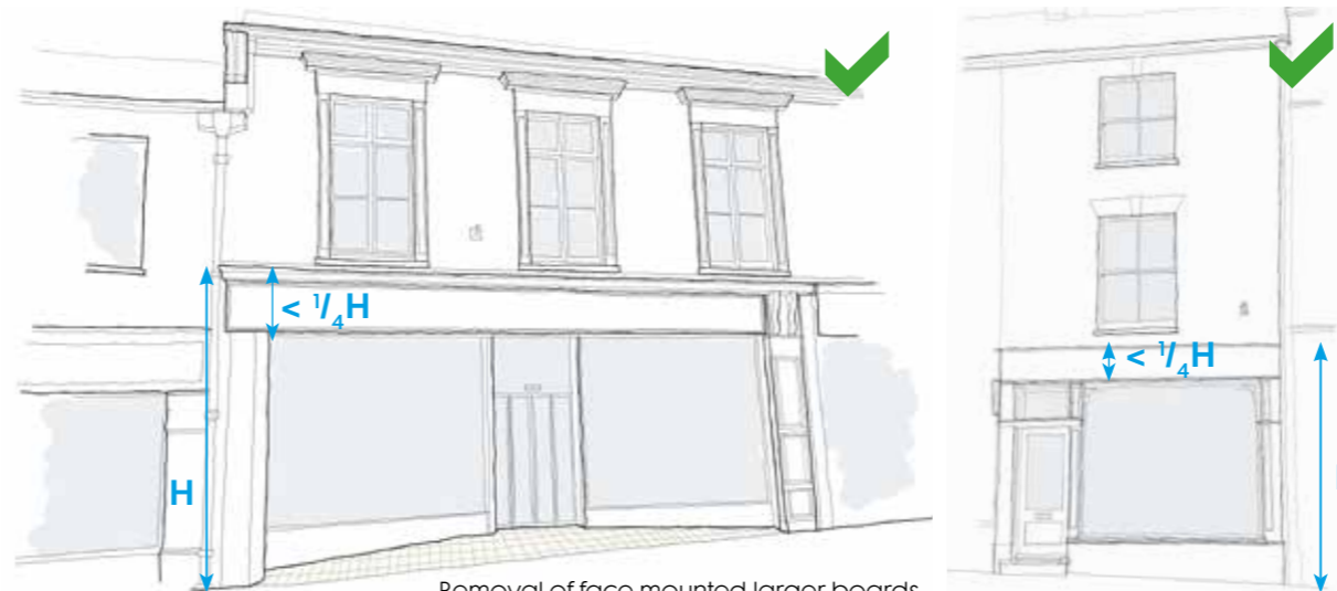
Removal of face mounted larger boards Allowing re-instatement of window heads, side pilaster details. Introducing cornice which offers protection from weathering above the sign
